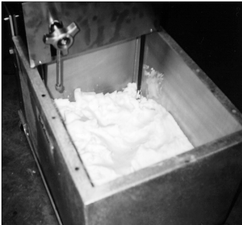
Figure 1-6. Packing Solid Shortening in the Kettle.
