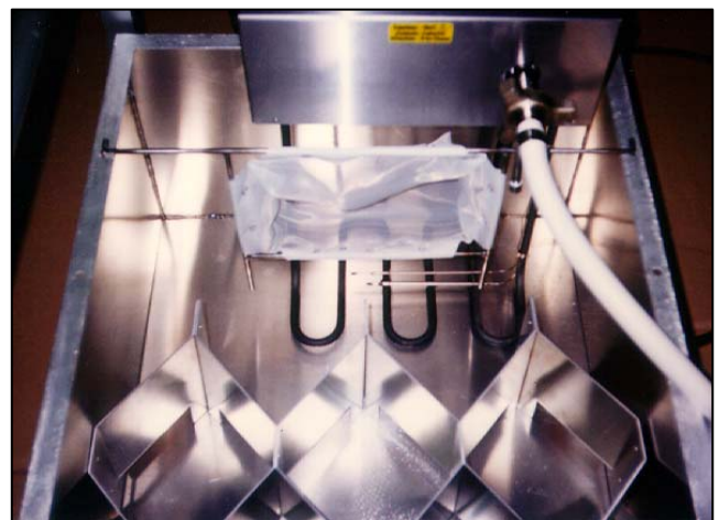
Figure 1-10. Positioning the Filter Frame for Melting.
