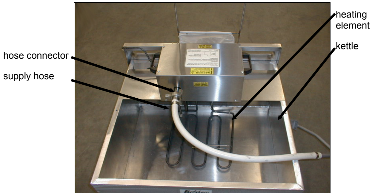
Figure 1-3. Top View, Heater Head.
