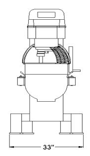
Electrical: 208/220 Volt 3 Phase 60 Hz 12 Amps 4 HP. Supplied with twist-lock plug.
