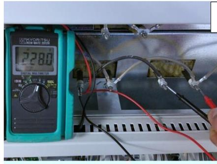
**11. Measure all heaters, there should be voltage on all heaters, top and bottom**
